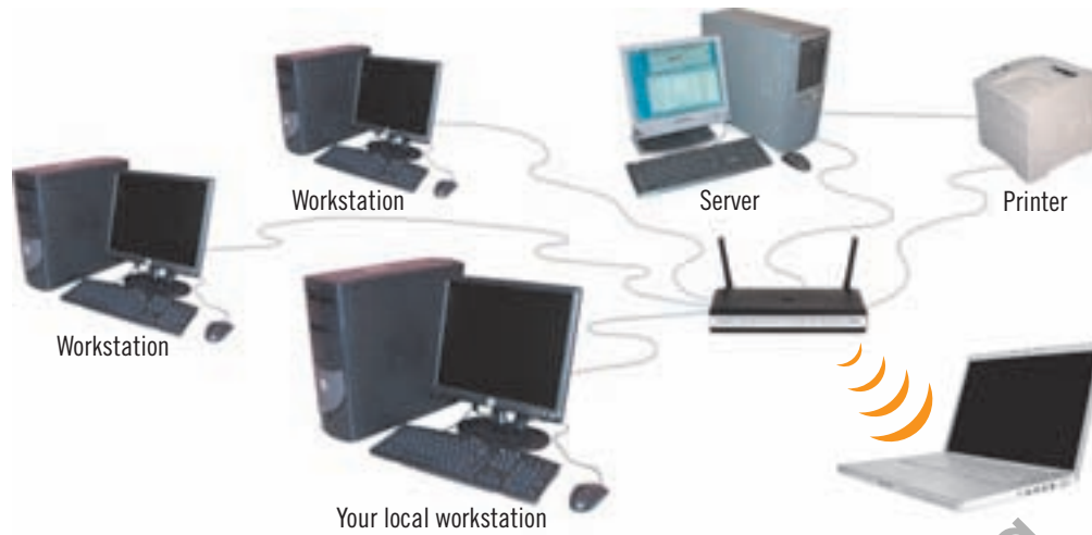
FIGURE A-18: Typical network configuration
